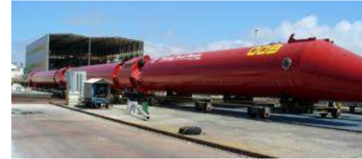
PELAMIS P2 pre-commercial model (2012) 180 m – 4 m diameter – 1350 t – 750 kW
